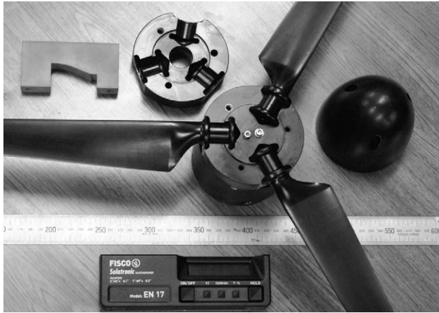
Fig. 1. Photograph of the blade and hub components.
